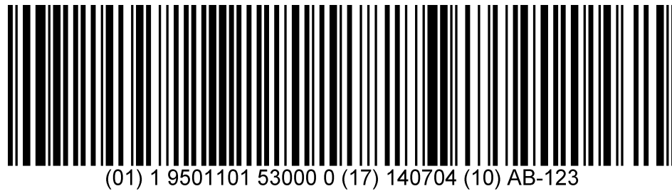
Figure 2-2 Example of a GS1-128 barcode representing a GTIN, a best before date, and a batch number
