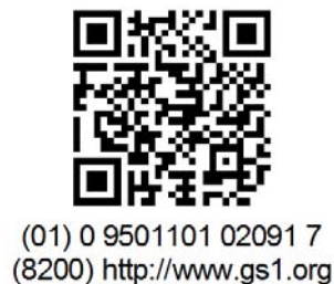
Figure 5-21 Example of GS1 QR Code symbol encoding a GTIN AI (01) and extended packaging URL: AI (8200)
