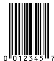
Figure 5.2.1.3.4-1. UPC-E barcode (encoding 001234000057 by zero-suppression)
